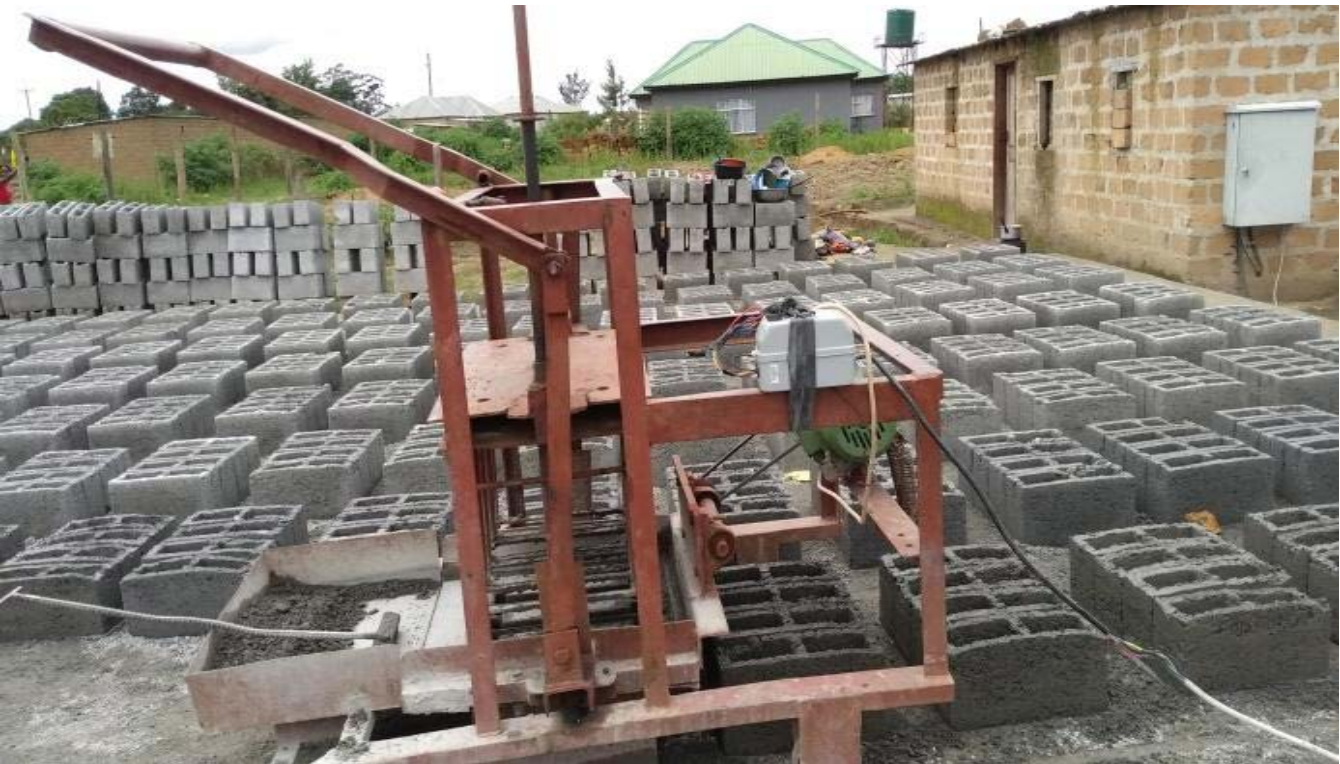
Figure 7: Production of 6" blocks being cured in readiness for marketing at the project site.
